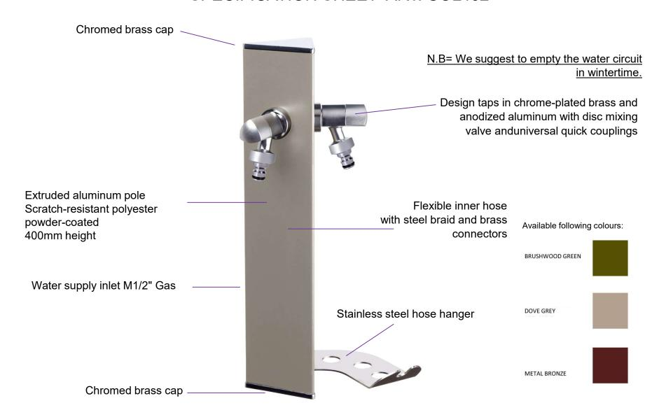
Working pressure 8 bar Water flow 15 l/m for each tap
